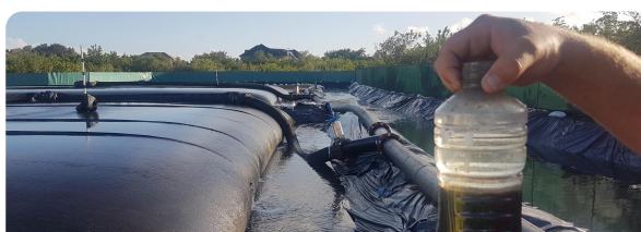
The result: clarified water at the foot of the tube
